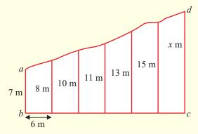
Using Simpson's Rule the area of the field is calculated to be  $410 \text{ m}^2$ . Calculate the value of x. [See Tables, page 42.]
