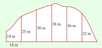
At equal intervals of 18 m along the dam, perpendicular measurements are made to the opposite bank, as shown on the sketch.
