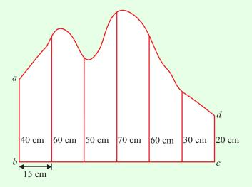
At equal intervals of 15 m along [bc], perpendicular measurements of 40 m, 60 m, 50 m, 70 m, 60 m, 30 m and 20 m are made to the top boundary.
