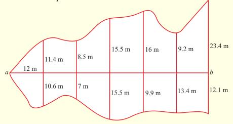
At equal intervals of 12 m along [ab], perpendicular measurements are made to the boundary, as shown on the sketch.
