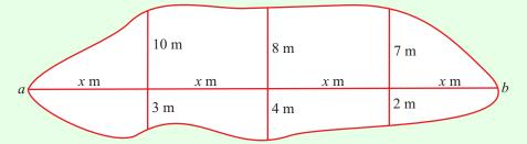
At equal intervals of x m along [ab] perpendicular measurements are made to the edges of the flood. The measurements to the top edge are 10 m, 8 m and 7 m. The measurements to the bottom edge are 3 m, 4 m and 2 m. At a and b the measurements are 0 m.
