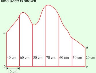
At equal intervals of 15 m along [bc], perpendicular measurements of 40 m, 60 m, 50 m, 70 m, 60 m, 30 m and 20 m are made to the top boundary.
