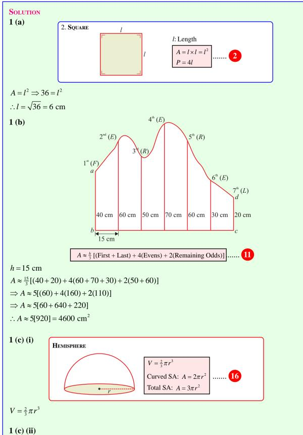
The tank is made up of 2 hemispheres (i.e. one sphere) and a cylinder. The radius of the cylinder and the sphere is the same.
